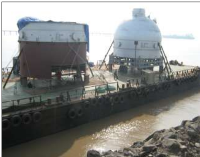
Package having dimension 10.17m X 10.17m X 6.90m – 168 MT and 206 MT loaded on our barge at Adani Dahej port jetty.
