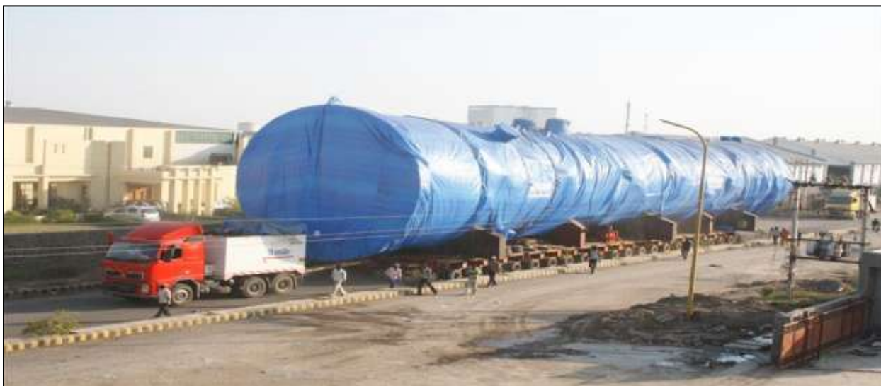
Main Fractionator 53.95m x 8.90m x 9.60m – 520 MT from Vijay Tank Kandla works to Kandla port
